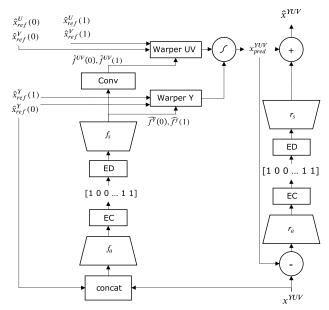
Figure 2. Coding structure for inter coded frames. The luminance component of the current frame as well as the reference pictures is used to derive the compressed motion information. At the decoder end, a strided convolution downsamples the motion flow to the resolution of chrominance before warping
