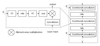
Figure 4. Convolutions / transpose convolutions with conditional activation in the autoencoders for residual and motion information.
