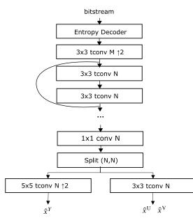
Figure 1. Example decoder architecture for YUV 4:2:0 output format (intra and residual).
