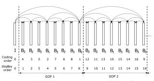
Figure 3. Prediction inter-dependencies in a sequence of two hierarchical GOP of 8 frames.
