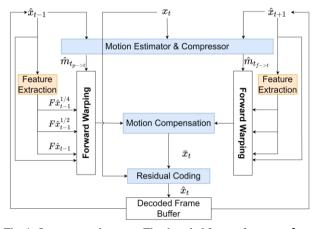
Fig. 1. Our proposed system. The decoded frames from past  $\hat{x}_{t-1}$ , and future  $\hat{x}_{t+1}$  are used in the motion estimator process to produce the motion vectors  $\hat{m}_{t_{p\to t}}$  and  $\hat{m}_{t_{f\to t}}$ .
