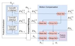
Fig. 2. We use forward warping to estimate the motion compensated feature/frame. Each of estimated frames is masked and merged using neural networks.
